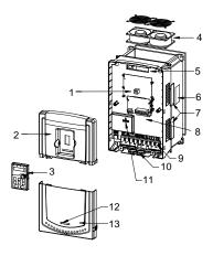
Figure 3-5 Product structure diagram
