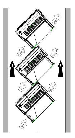
Figure 4-5 Tilt installation
