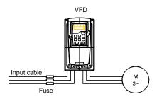
Figure 4-25 Fuse configuration
